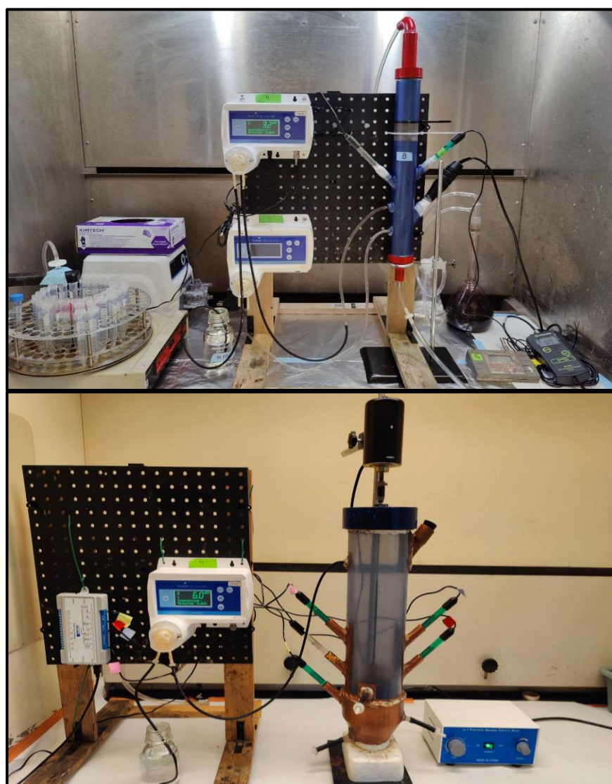
Figure 6 - Two types of laboratory scale ME reactors: 500 mL reactor (top), 3 L reactor (bottom) Further details on the equipment, materials, and chemicals are provided in the next section.
