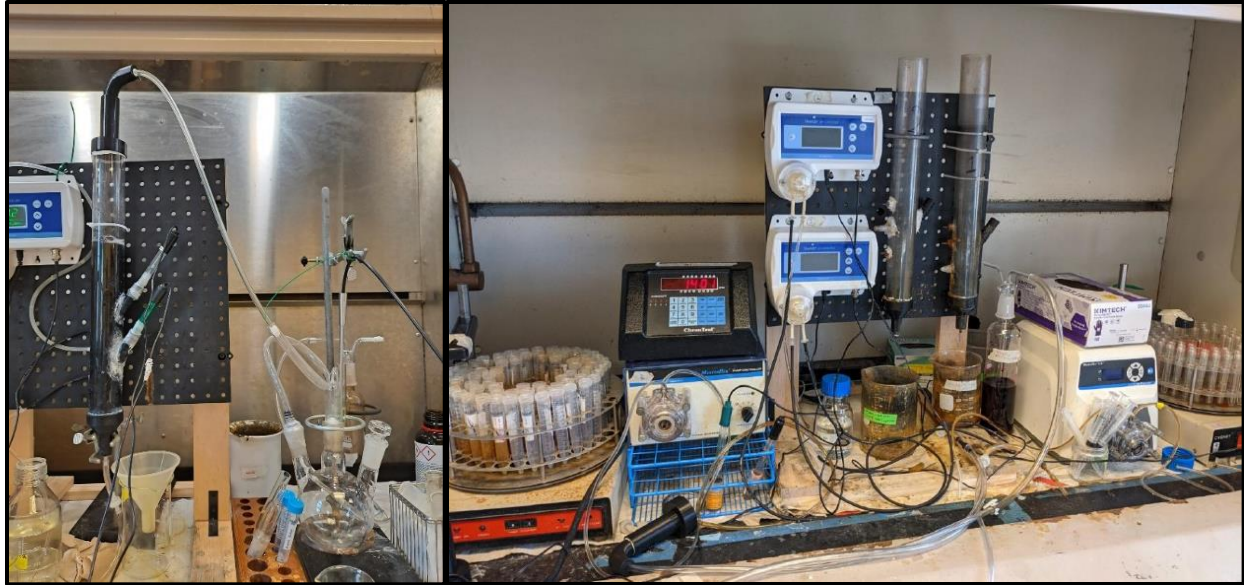
Figure 10 - 500 mL column reactor used for ME experiments at the beginning of phase III
