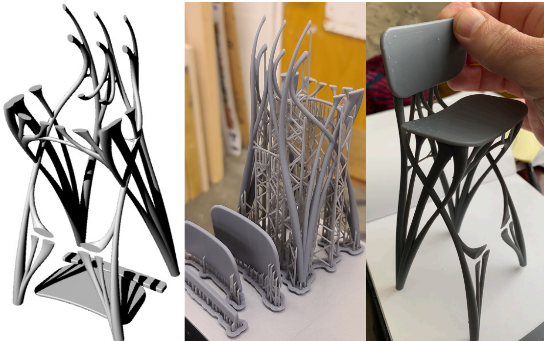
Image 4.3.3.15 From left to right: preparing a file for 3D SLA printing, a finished print with support structure, validating designs with a tangible prototype
