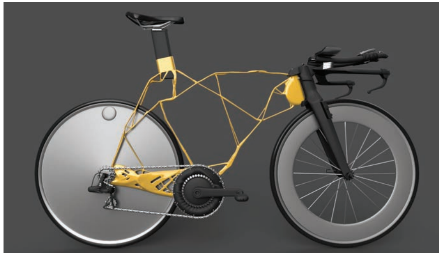
Image 3.6.3.1 A generatively produced bike frame [76]
