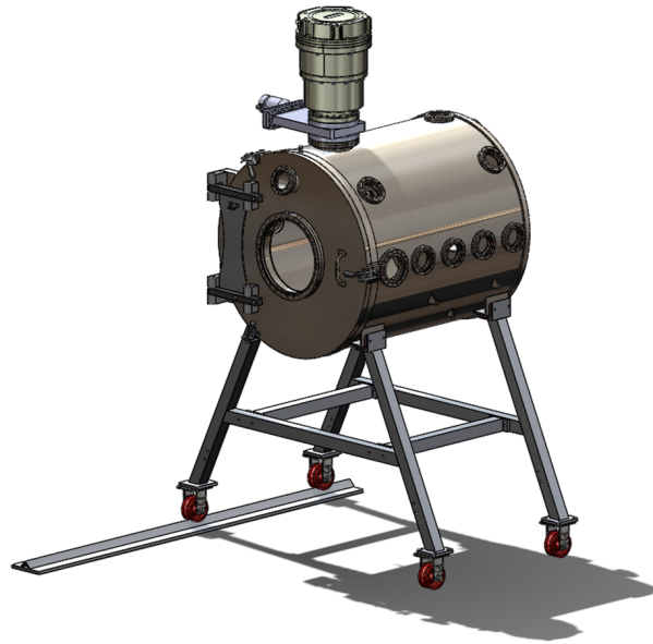
Figure 5.5: The Exhaust Chamber frame is guided by a rail. The chamber can be removed from the ZaP-HD device without use of a crane, improving safety while reducing the time required to maintain or repair the device.
