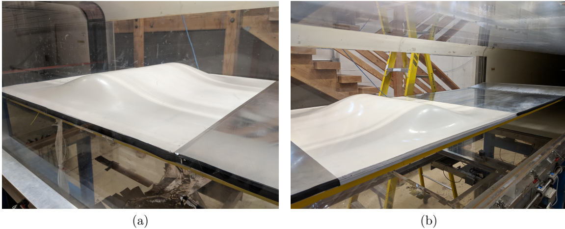
Figure 3.8: Three-dimensional bump integrated into tunnel and splitter plate from (a) Looking upstream. (b) Looking downstream.
