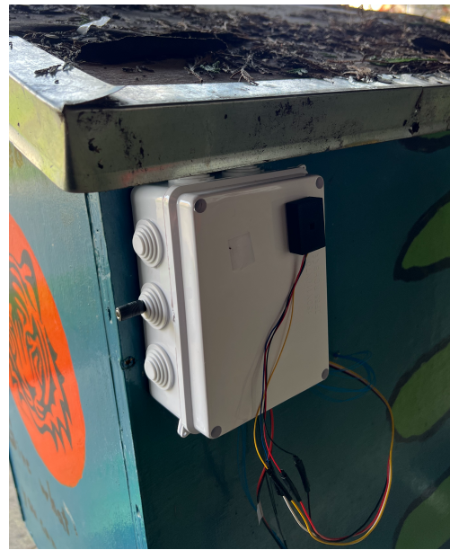
(b) Enclosure mounted inside pantry with BME688 sensor installed externally for environmental monitoring.
