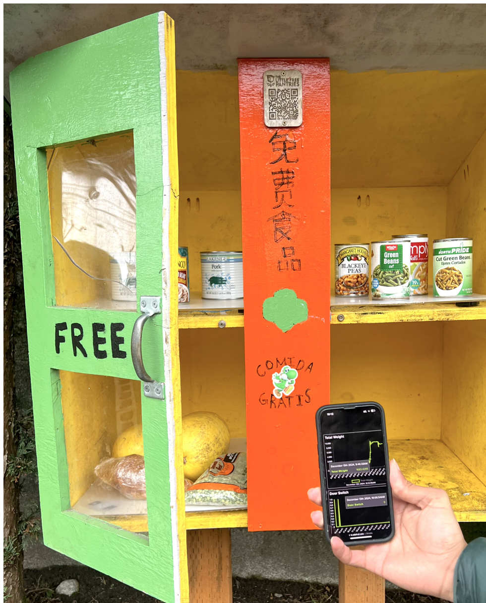
Figure 5.1: Deployed micro-pantry at the Seattle pilot site with real-time monitoring displayed on a mobile device via Adafruit IO dashboard
