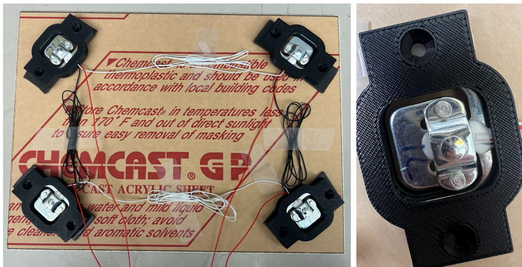
(a) Arrangement of load cells in Wheatstone bridge configuration beneath acrylic shelf. (b) Close-up of load cell mounted in 3D-printed case.
