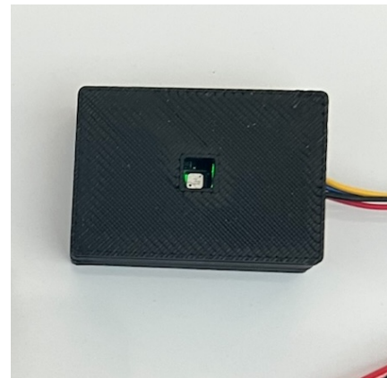
(b) BME688 installed in a 3D-printed enclosure for protection
