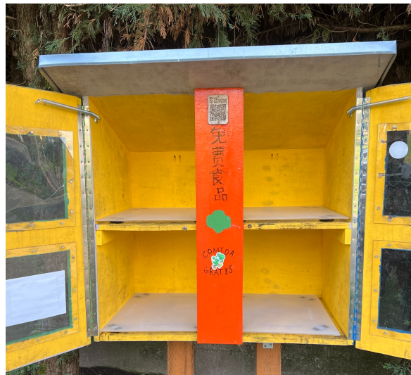
(c) Fully installed micro-pantry with shelves and weight sensors
