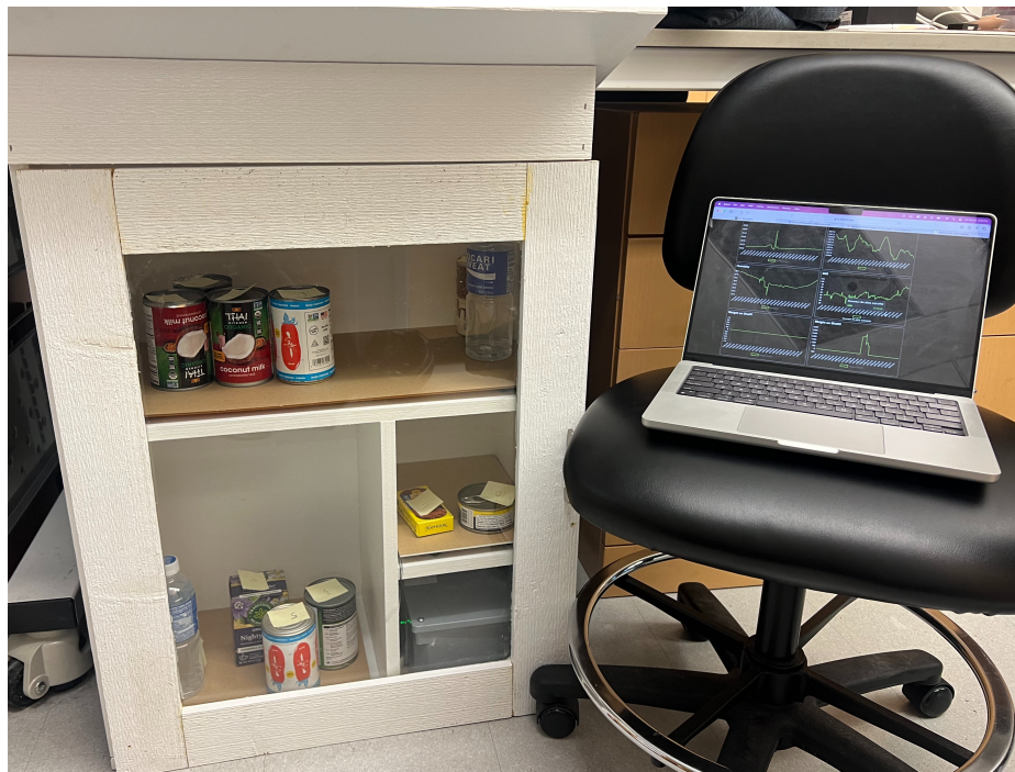
Figure 5.4: Example Adafruit IO dashboard visualization of shelf weight, door activity, and temperature during lab test
