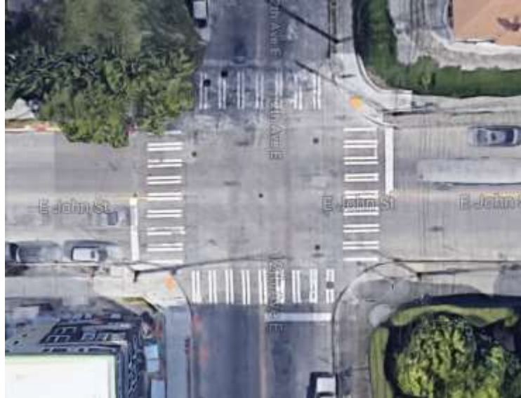
Figure 6 Aerial image of intersection at 12 th and John showing lane configuration (Google 2019)
