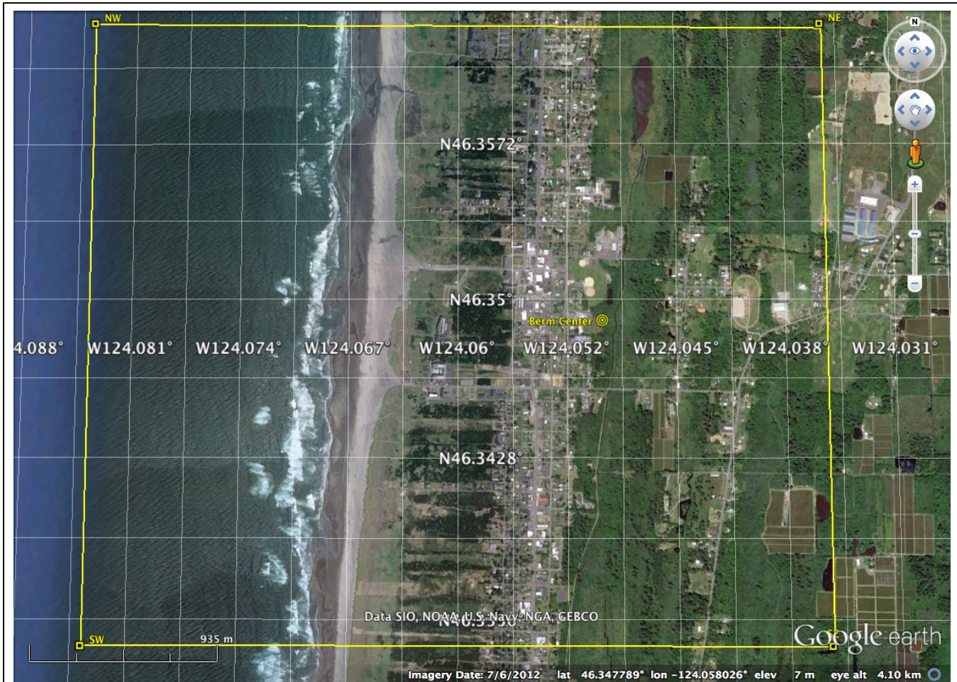
Figure 2. Google Earth image of the Long Beach area. The yellow lines mark the geographical extent of the 1/3 arc-second DEM developed for this study by WA DNR, using the 1-m resolution Lidar data collected for DOGAMI in 2009 (DOGAMI, 2010), and the yellow bulls-eye symbol marks the location of the proposed berm.
