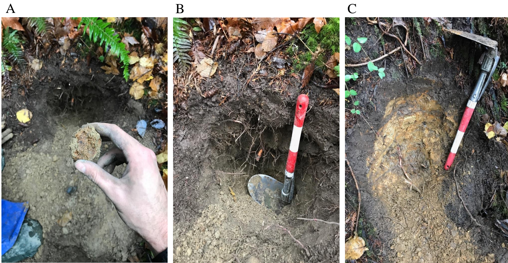
Figure 28: A) Example of a test pit where saprolitic bedrock was found at the base of the pit in the form of core stones. B) Example of a test pit where till and/or colluvium was found throughout the entire depth of the pit. C) Example of a test pit where a thin veneer of soil/colluvium covered bedrock.
