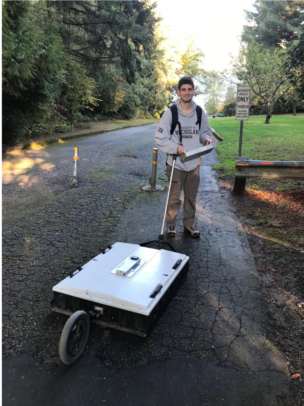
Figure 13: Author shown with the MALA GX 80 MHz GPR instrument. This was the ground-penetrating radar system used in the geophysical investigation.
