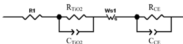
Scheme 2: Electrical equivalent circuit of the DSC under illumination at Voc 49
