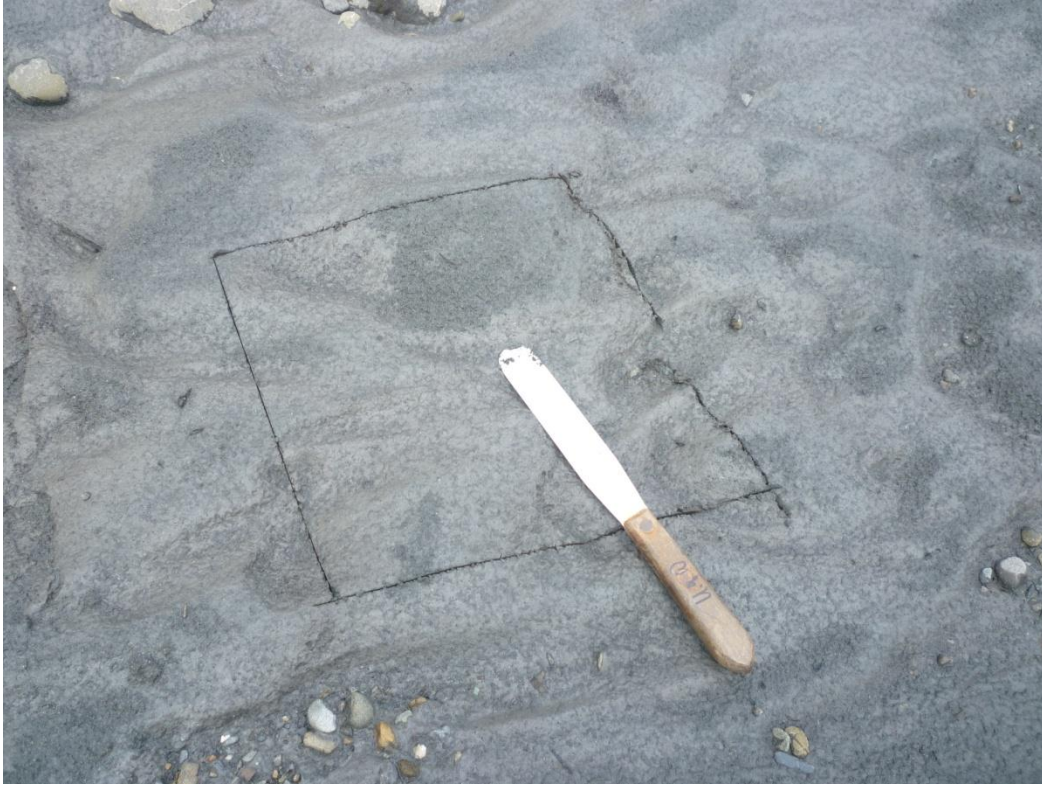
Figure 2. Surface scrape sample measuring a cross-section of 20 cm × 20 cm and scraping off the first cm of sediment. Elwha River, former Lake Mills, WP 175.
