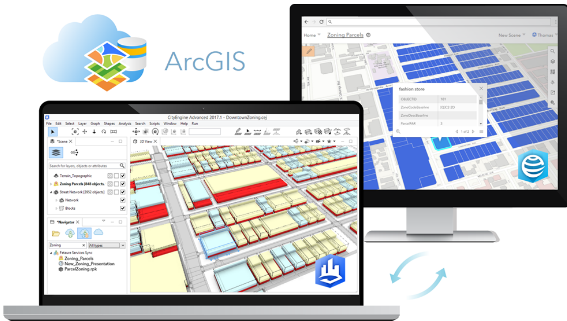
Figure 95. Example of integration between systems supporting advanced design capabilities like rule-based design generation (block-scale massing based), and more generalized design representation (2-D zoning layer). Here zoning polygons can be updated in AGOL (or using other Esri tools like GeoPlanner) and replicated to City Engine.
