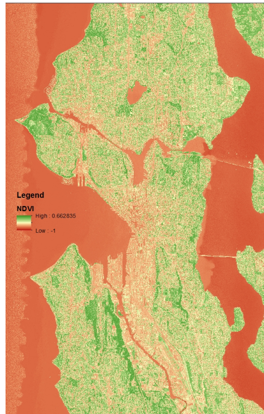
Figure 12. Seattle's NDVI calculated from NAIP imagery (1m 2 resolution) using ArcGIS Desktop image analysis. Based on a threshold of .06 for vegetation, Seattle is 38% vegetated. NAIP source: USDA ArcGIS Server. NDVI and map source: Author.
