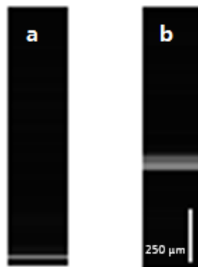
Figure 22. 1D depth images for a gold coated mirror surface (A-scan only) for 1V galvanometer scanning. Left, zero position, right, 25 \mu\text{m} further away from zero position
