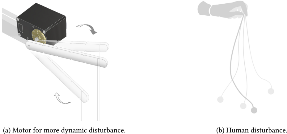
Figure 6.10: Dynamic disturbance evaluations we considered. These disturbances test the robustness of the learned CherryBot policies.
