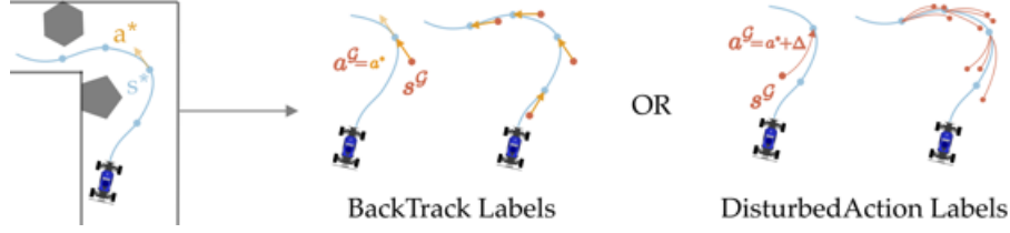
Figure 5.3: Generating corrective labels from demonstration. Given expert demonstration state s^* and action a^* that arrives at s_{next}^* . BackTrack Labels: search for an alternative starting state s^G that can arrive at expert state s^* if it executes expert action a^* . DisturbedAction Labels: search for an alternative starting state s^G that would arrive at s_{next}^* if it executes a slightly disturbed expert action a^G = a_t^* + \Delta , where \Delta is a sampled noise.
