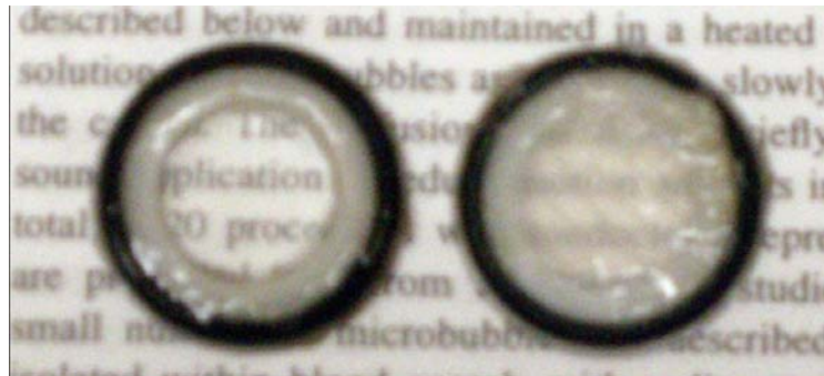
Figure 2.1 Comparison of rat mesentery (left) and cecum (right) tissues. Tissue samples were captured by holders with O-rings and put on a piece of paper. Mesentery tissue has better optical transparency than the cecum.
