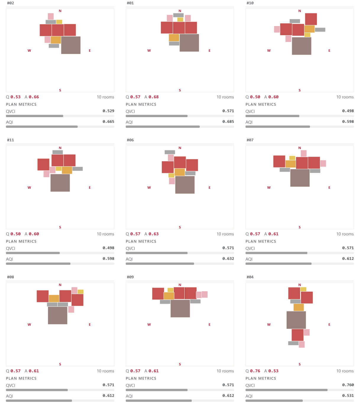
Figure 4.3: Generated schematic layouts for the same plan with the acoustic target raised to AQI = 0.70 (view target held at QVCI = 0.50). The achieved AQI of the leading candidates rises to as high as 0.685, while a high-view candidate (QVCI 0.760) is still produced.
