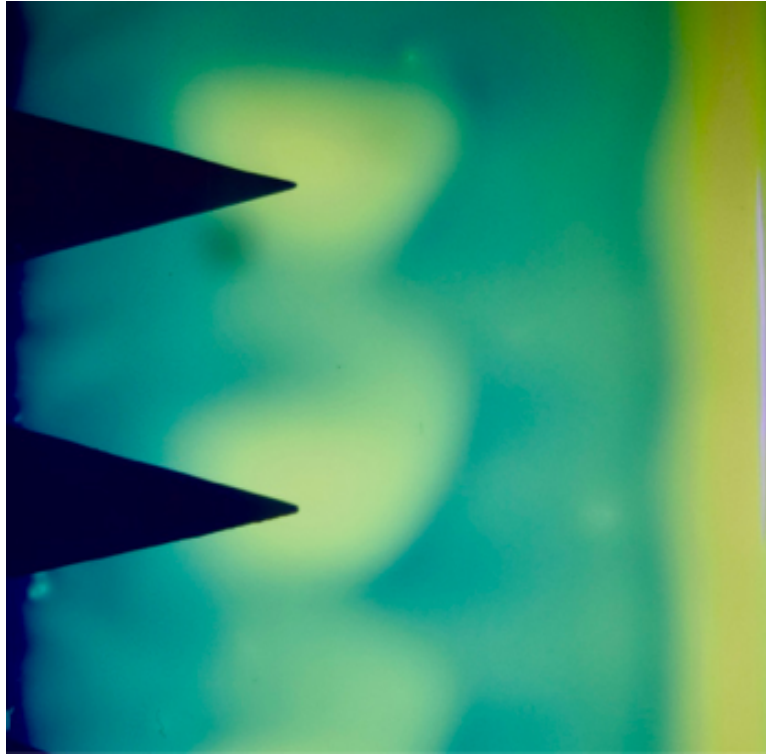
Figure 3.6: Flow visualization of the sharp delta devices at \xi = 1.00 , \eta = 0.16
