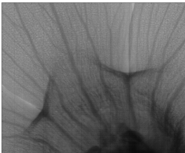
Figure 7.3: (a) Radiograph of a flower petal. The grayscale is a representation of raw incident intensity. Improved spatial resolution would be achieved by selection of single-pixel events. (b) X-ray emission spectrum of a Mn metal foil excited by a low-power laboratory x-ray tube source. The spectrum is based only on nominally single-pixel events.
