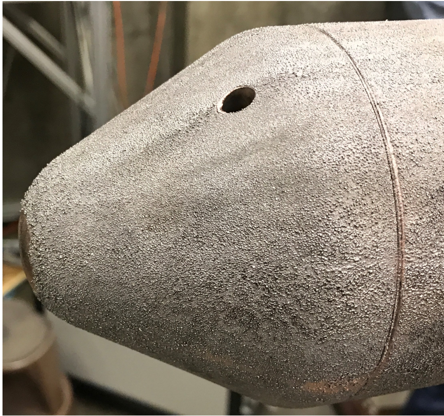
Figure 3.1: The tungsten-sprayed copper nose cone during disassembly of the ZaP-HD device. The tungsten at the tip has been completely eroded, exposing the bare copper underneath.
