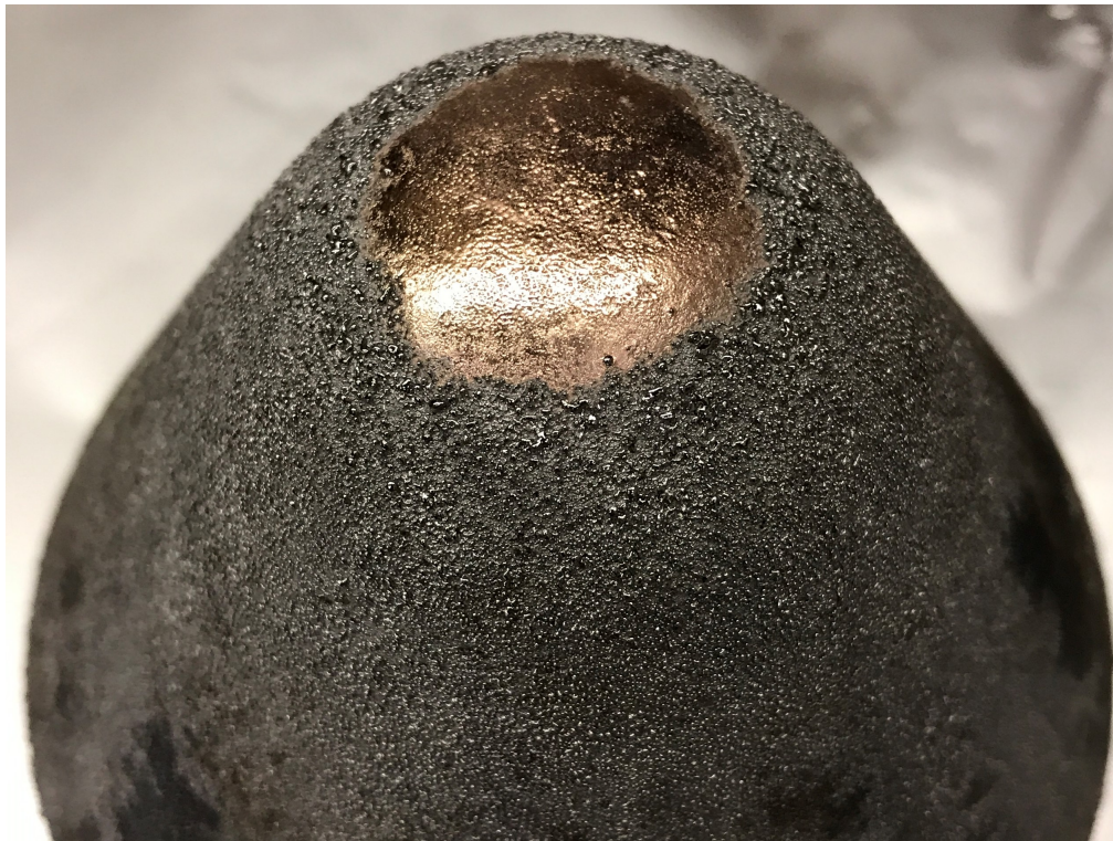
Figure 3.2: The region of tungsten erosion is approximately one inch in diameter. The copper surface has been roughened by the pits and craters that have formed. Molten tungsten cooled and formed droplets which can be seen at the periphery of the exposed copper. The size of the droplets decreases away from the tip.
