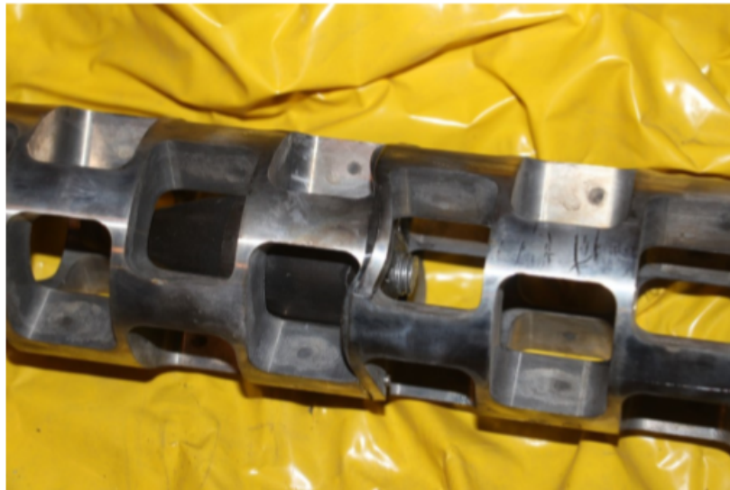
Figure 3.6: Yielded insert with local failure; Broken and lodged projectile
