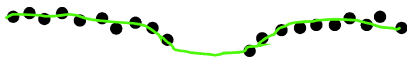
Figure 20. Example of a cloud of points at a concavity with low point density, and the corresponding surface generation
