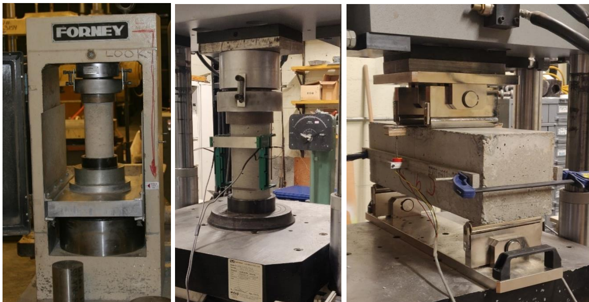
Figure 3-5: Material Testing (a) Compressive Strength (b) Compressive Modulus (c) Flexural Strength and Toughness
