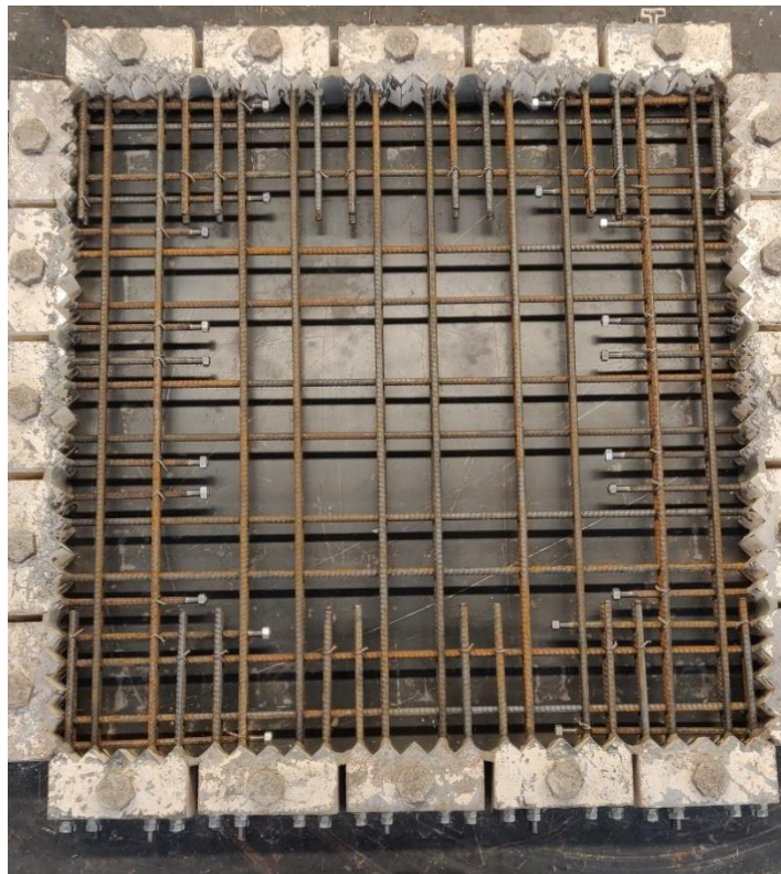
Figure 3-3: Panel Form Ready for Cast
