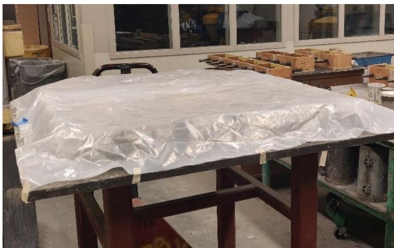
Figure 3-4: Panel Specimen Curing
