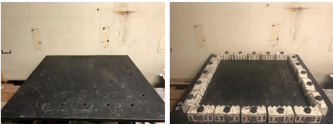
Figure 3-2: Casting Table with and without Shear Keys
