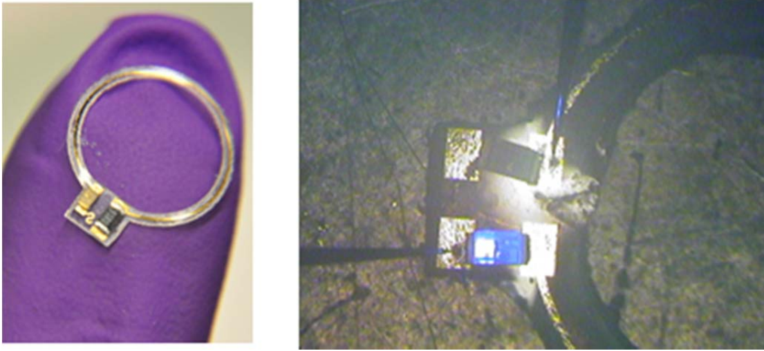
Figure 2.8: Left: Assembled device (actual chips replaced with SMT devices with dimensions similar to the chips for testing the packaging method). Right: Illuminated LED showing the conductivity of the metal pattern.
