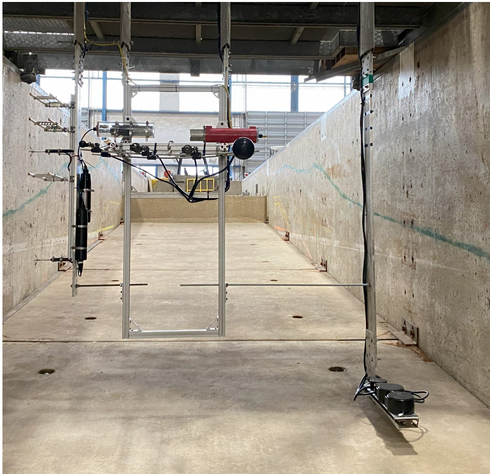
Figure 2.4: Image of the front of our in-situ instruments. The instruments are attached to vertical farings that can be lowered or raised together. From the left structure (from top to bottom), the instruments are two void probes, one ADV, one void probe, and one ADV. The center structure, connected to two farings, has a light source and bubble camera in water housing units and the acoustic velocity and attenuation system. The faring on the right has upward-facing echosounders.
