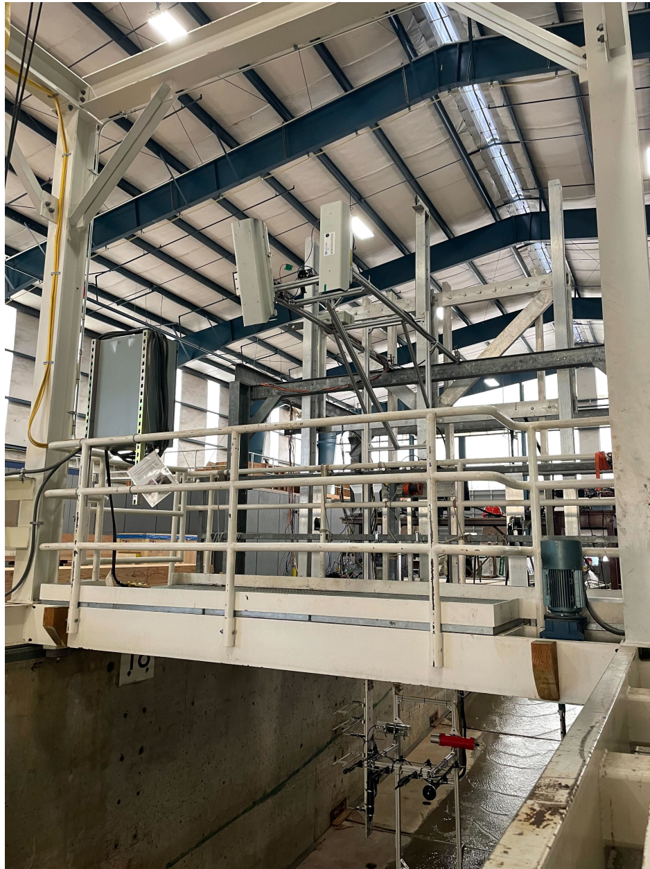
Figure 2.3: Image of the two carts on top of the walls of the flume. They ride above the tank to allow for instruments to be deployed into the flume at different locations and depths. The white cart is motorized to move along the tank. The instrument cart (behind the white cart in this view) is not motorized but can be pushed by the white cart to move along the tank. Two structures were mounted onto the instrument cart: one structure was used for top-view instruments, looking down into the flume and one structure was mounted onto fins to lower instruments into the water column.
