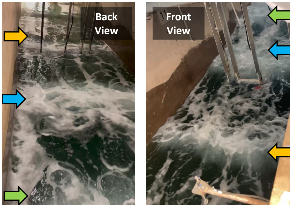
Figure 4.6: Images of after wave breaking of instrumentation at Location 4. The left image is a back view of the instrumentation. The right image is a front view of the instrumentation. These images were taken of different runs. However, the locations of the bubble plume injection are similar for each run. Corresponding arrow colors are similar locations of bubble injection.
