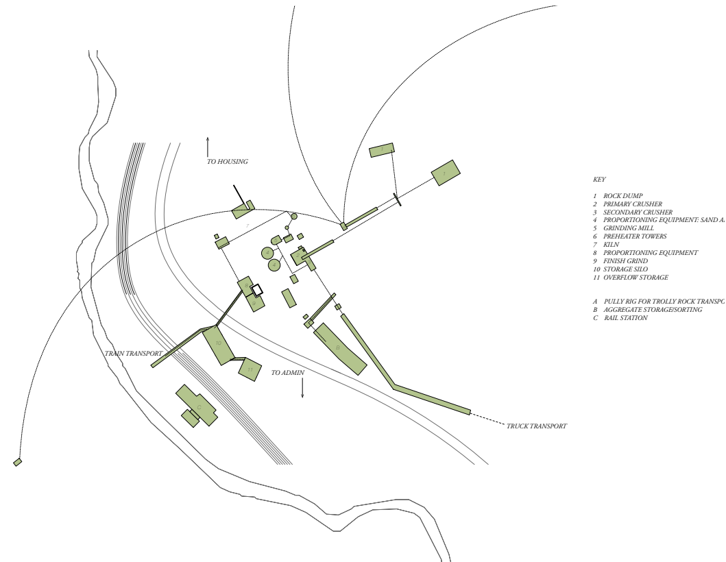
58 Mining the site: Structures were placed based on efficiency of moving material
