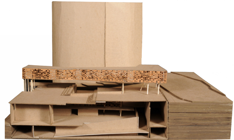
FIGURE 88 Photo of building section with the model pulled apart to reveal the section
