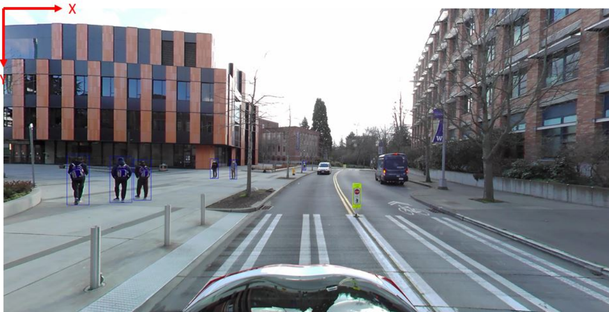
Figure 3.2: Pedestrian detection with bounding boxes and coordinate axes.
