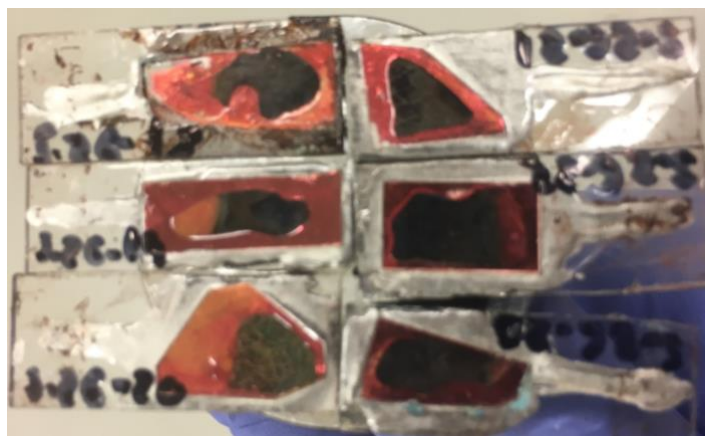
Figure 14: Templates after deposition showing darkened areas of nanowires
