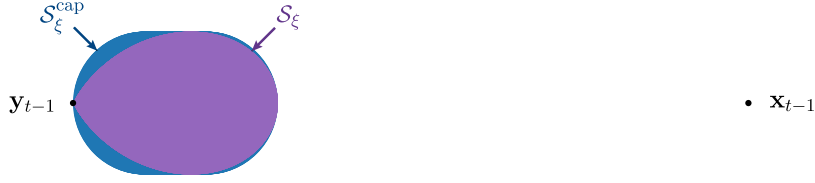
Figure 3.4: Capsule approximation. To simplify computation, BlitzMN constructs \mathcal{W}_t using \mathcal{S}_\xi^{\text{cap}} , which is a relaxation of \mathcal{S}_\xi . \mathcal{S}_\xi is shaped like a teardrop when \xi_t is small, while \mathcal{S}_\xi^{\text{cap}} is the smallest capsule (convex hull of two balls with equal radius) that contains \mathcal{S}_\xi . For the figure, \xi_t = 0.4 , and \|\mathbf{x}_{t-1} - \mathbf{y}_{t-1}\|^2 / \Delta_{t-1} = 1 .
