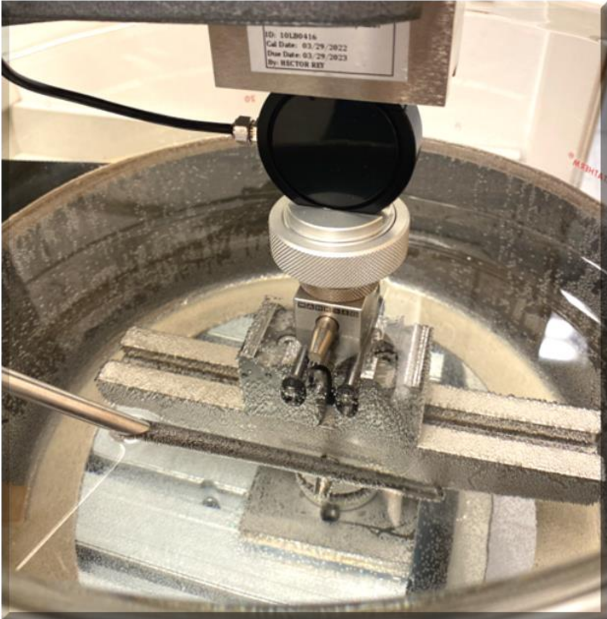
Immersion of the thermoformed plastic in the water bath
