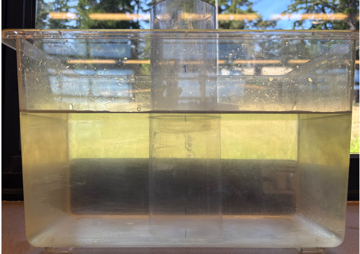
Figure 2: Treatment tank and acclimation tube. The treatment tank was 16.5cm x 30.5cm x 21.6cm. The tube was 27.5cm tall and had an internal diameter of 8cm. The tank was filled with 6L of filtered seawater prior to each trial.
