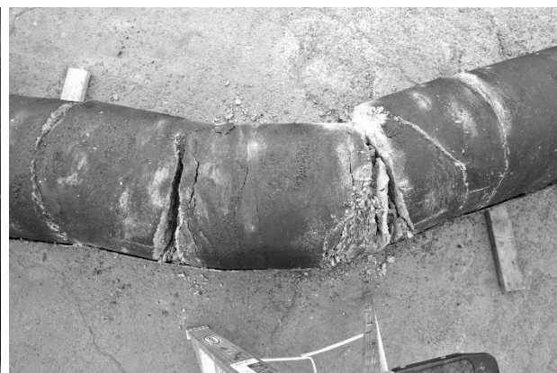
f) Specimen 9 concrete cracking
