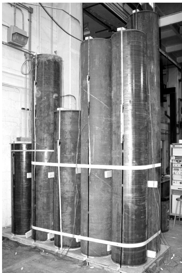
Figure 3.18: Specimen casting support
