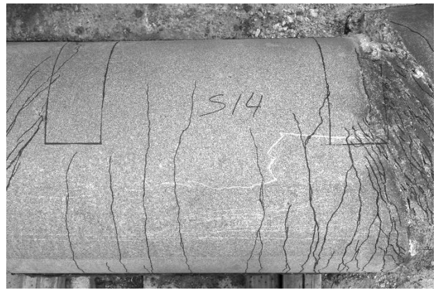
d) Specimen 14 mid-span concrete cracking
