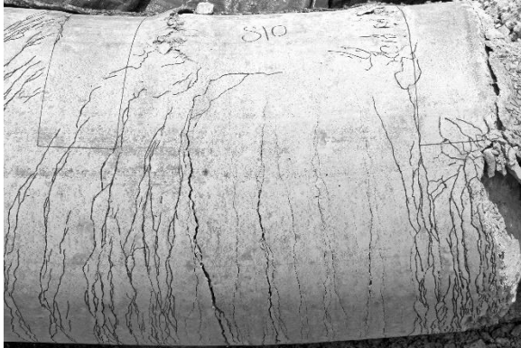
Figure 5.9: Dense flexural cracking
