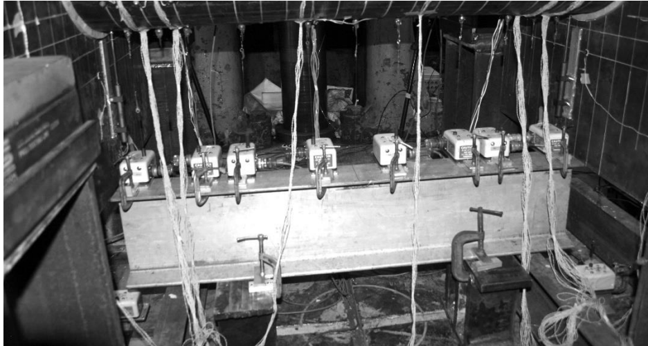
Figure B-11: String pots—west
