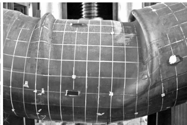
d) Specimen 9 steel buckling
