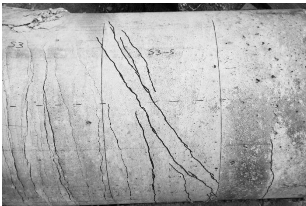
f) Specimen 3 south span concrete cracking
