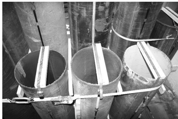
Figure 3.17: Specimen casting support
