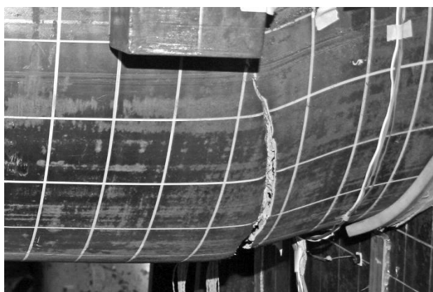
c) Specimen 16 steel tear
