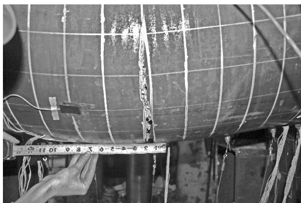
c) Specimen 2 steel tear
