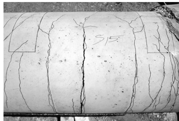
d) Specimen 15 mid-span concrete cracking
