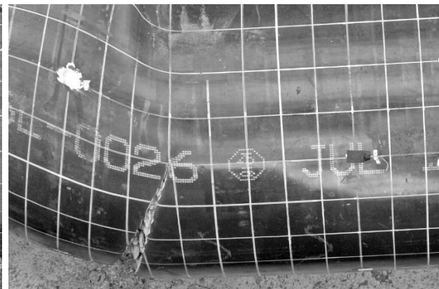
Figure 5.5: Inclined steel tear
