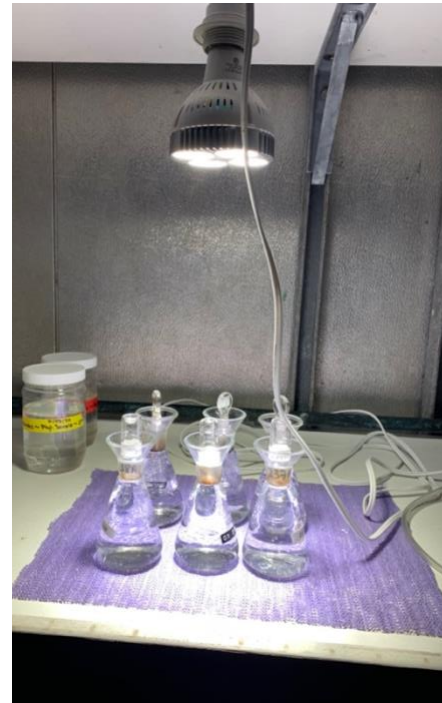
Figure 3. Light bottles in the in-situ incubation room with light shining on them for the whole incubation time.
