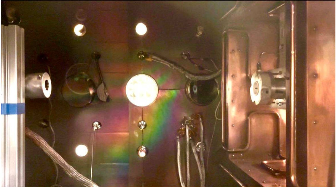
Figure 18: Installed RPA Relative to Thruster
