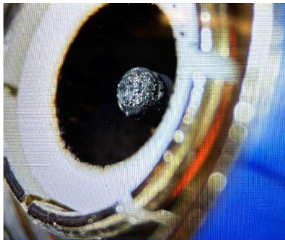
Figure 6: TNC Char Buildup from PTFE Ablation
