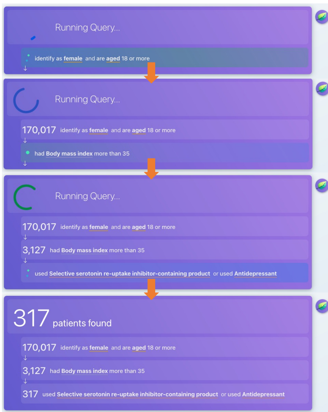
Figure 8.3: A time-lapse representation asynchronously reporting of incremental query results, from top to bottom. This is performed using two streaming interfaces, one from the clinical database to the API, and a second from the API to the web application.
