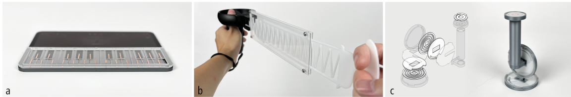
Figure 6.1: Example applications made with FlexHaptics method: (a) a piano keyboard interface for touchscreen musical applications, (b) a VR controller attachment for bow shooting games, and (c) a joystick with a two-step button on the stick end.
