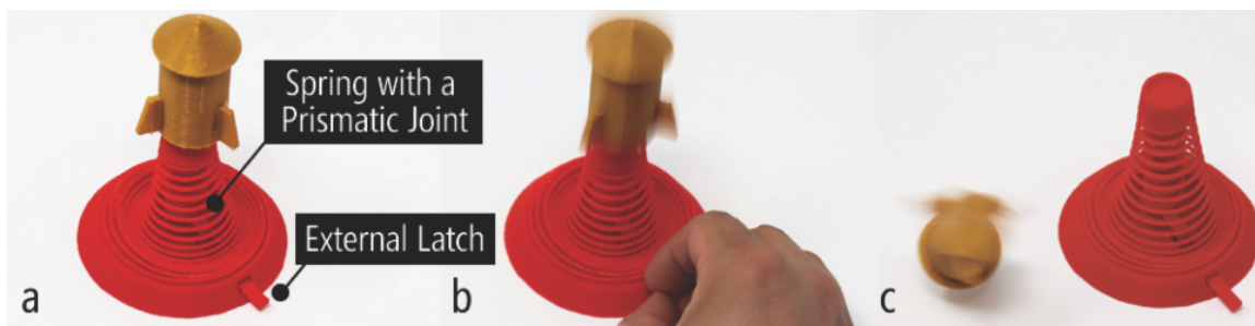
Figure 4.18: A launching rocket application: (a) a rocket sits on top of a compressed “smoke” spring, which is locked by an external latch; (b) the user can launch the rocket by pulling the latch; and (c) the smoke is in its full extension.
