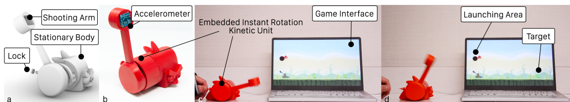
Figure 5.12: A catapult-like game controller is made to virtually projectile birds in an Angry Birds game: (a) the rendered 3D model of the game controller, (b) the printed game controller with external sensor and circuitry embedded, (c) flying the bird at a small angle, and (d) flying the bird at a bigger angle.
