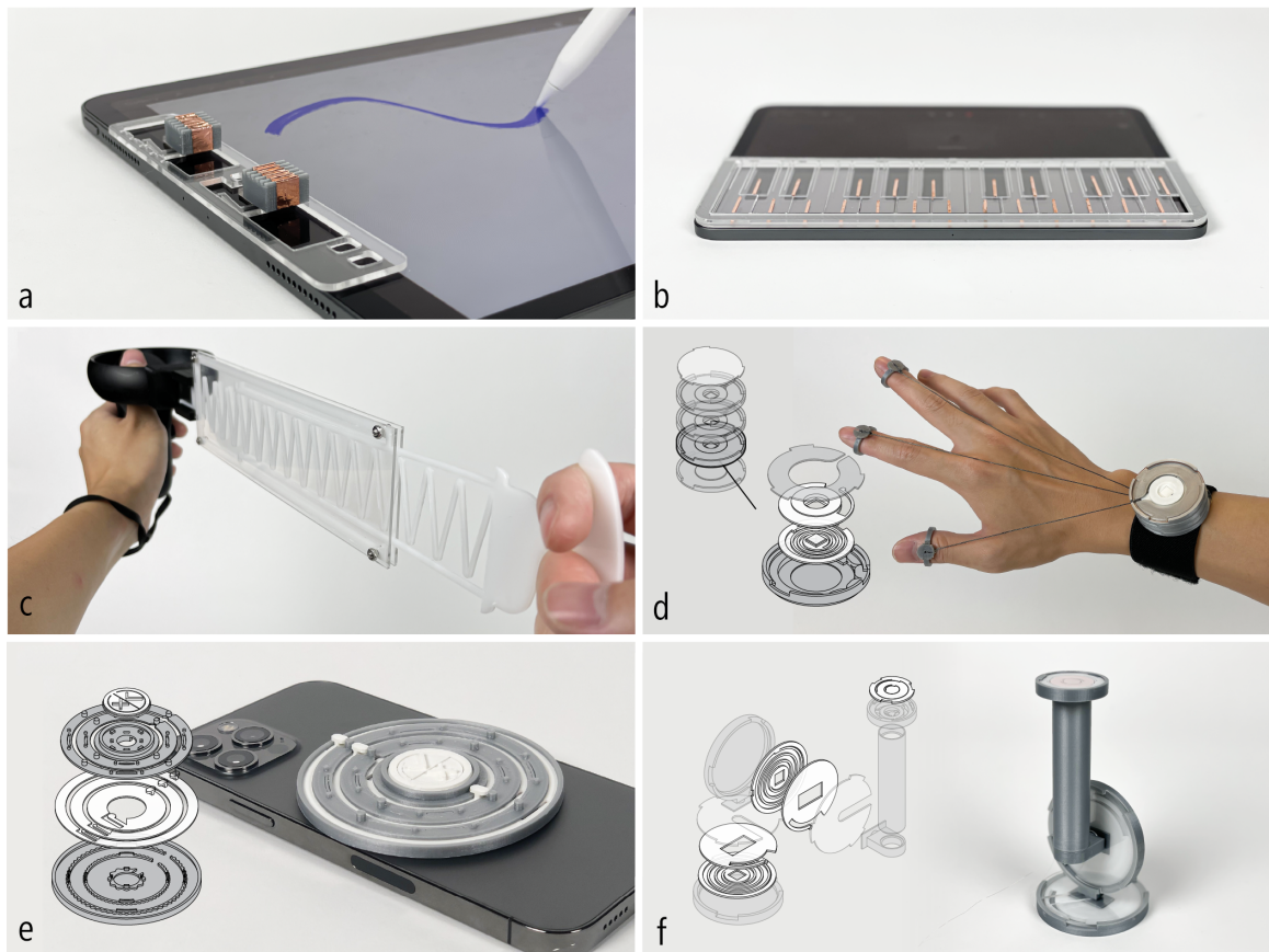
Figure 6.10: Application examples: (a) a slider input interface for touchscreen painting applications, (b) a piano keyboard interface for touchscreen musical applications, (c) a VR controller attachment for bow shooting games, (d) a string-based wearable haptic device, (e) a tactile low vision timer, and (f) a joystick with a two-step button on the stick end.
