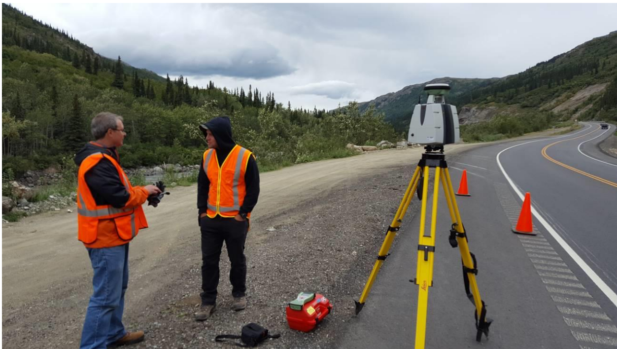
Figure 4.2 Example terrestrial laser scan set-up with the Leica P40 at a Glitter Gulch site.
