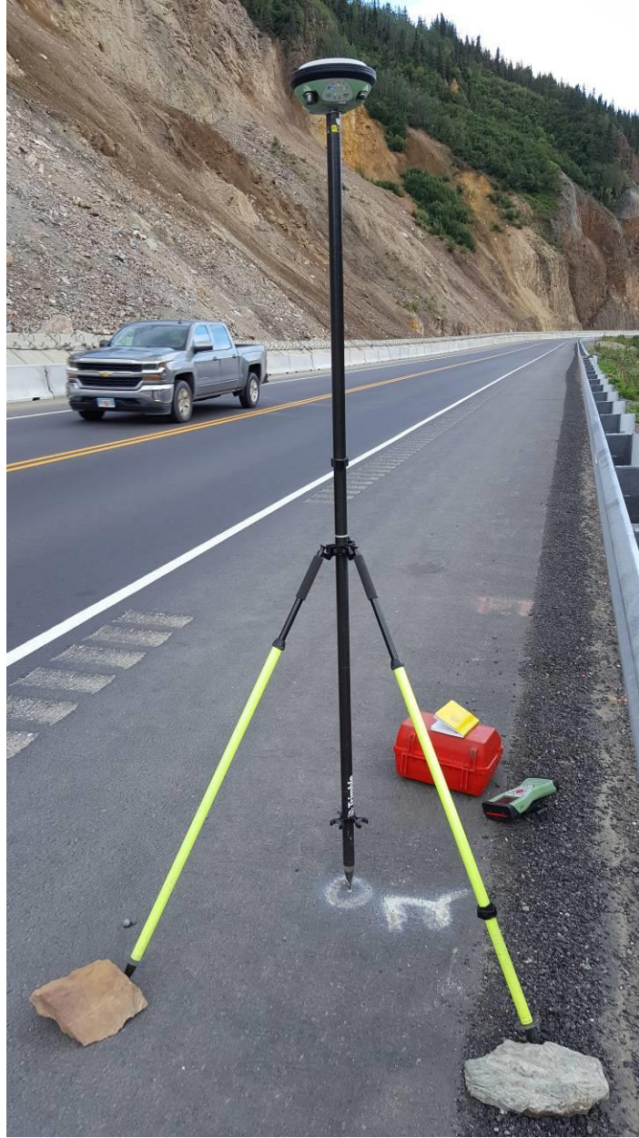
Figure 4.4 Example GNSS survey observation on a ground control point used to provide georeferencing information for the total station.
