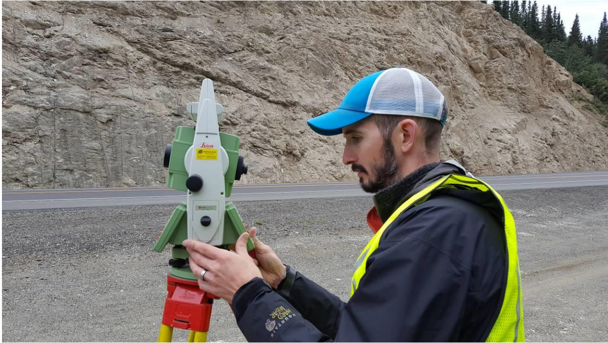
Figure 4.3 Example operation of the total station at a Glitter Gulch site to acquire reflectorless measurements on the cliff face.
