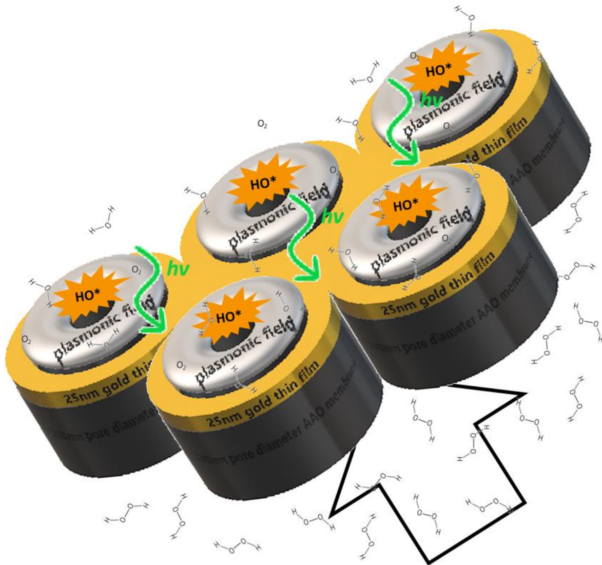
Figure 4.1. Schematic of Au@AAO membrane with generation of \text{HO}^* radicals via flowing \text{H}_2\text{O}_2 solution through plasmonic membrane with plasmonic activation at pore exits with 25nm thick layer of gold.
