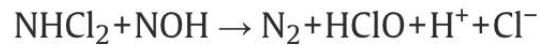
Figure 1.8. The proposed photocatalytic reactions and pathway for the ammonia nitrogen removal by the PEC-chloride system; reproduced with permission from ref [50]. Copyright 2017, Elsevier.
