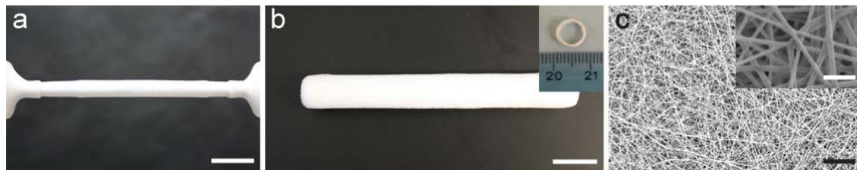
Figure 8.9: Tubular scaffolds with randomly oriented fibers prepared by electrospinning CS/PCL solution. (a) Photograph of the tubular scaffold deposited on cylindrical conductive electrode (scale bar: 1.5 cm). (b) Photograph of the tubular scaffold removed from the electrode (scale bar: 1 cm). Inset: photograph of the cross-section of the tube with an inner diameter of \sim 7 mm. (c) SEM image of randomly oriented fibers in the tube (scale bar: 5 \mu\text{m} ). Inset: image of fibers at higher magnification (diameters of fibers: 120–180 nm, scale bar: 1 \mu\text{m} ).
