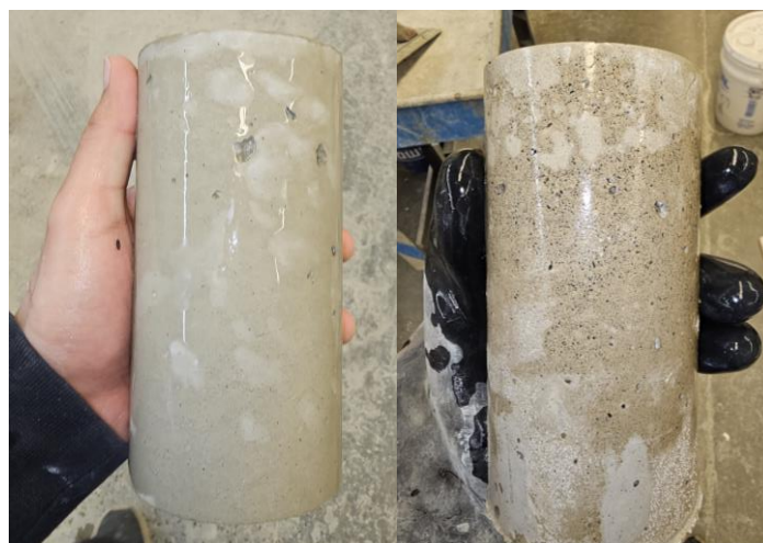
Figure 3.17: Etching Observed on Cylinders Cured in Normal vs Oversaturated Lime Bath
