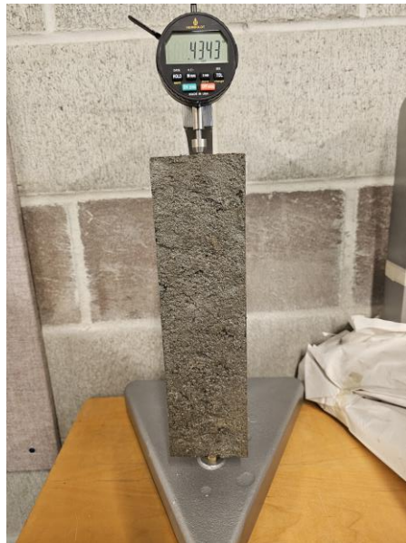
Figure 3.24: Drying Shrinkage Beam Sitting on Comparator
