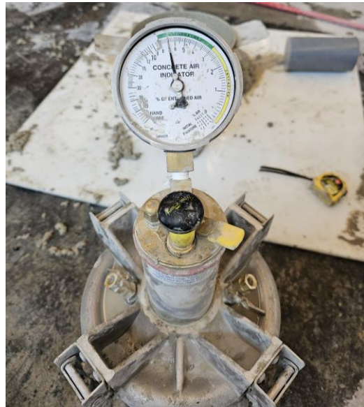
Figure 3.19: Air Content Testing of CSA As-Is Concrete Mixture
