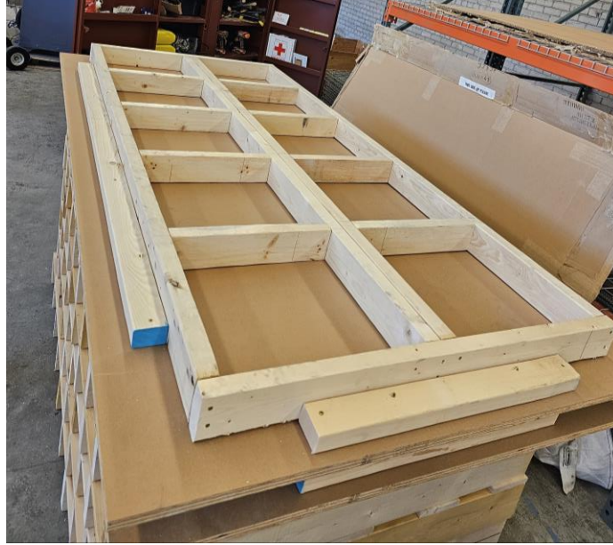
Figure 3.4: Paver-Sized Substrate Formwork.
