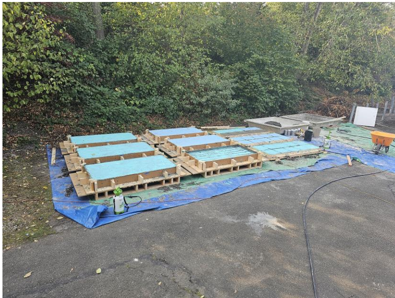
Figure A.14: Top-Surface Retarders Applied
