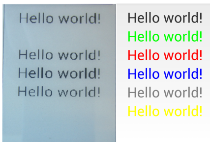
Figure 13.3: Displaying differently colored text. The e-paper display image (left) and the original phone screenshot (right). The green and yellow text disappear when converted to e-paper format.
