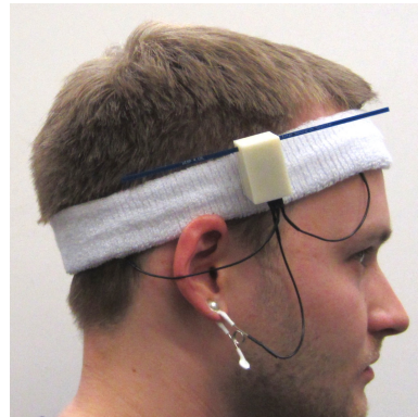
(b) Possible usage scenario. EEG-WISP is in a white plastic box. Black wires attach to the DRL and two electrodes, placed under the white headband.
