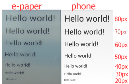
Figure 13.2: Displaying different font sizes. The e-paper display image (left) and the original phone screenshot (right)
