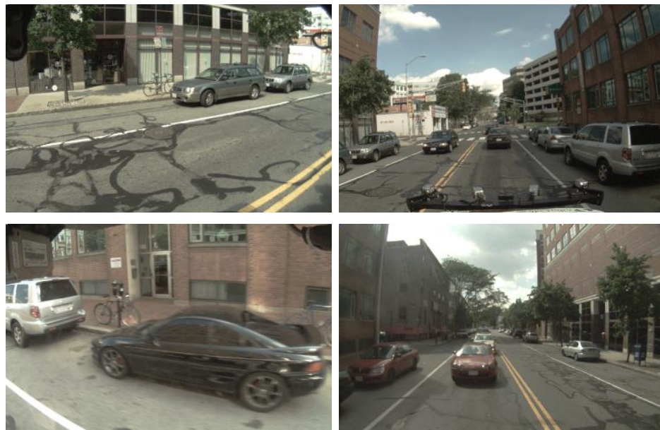
Figure 4.4: A scene from the urban driving data set. Starting with the image in the top left and going clockwise, they are captured with left-, forward-, right-, and rear-facing cameras mounted on the vehicle.
