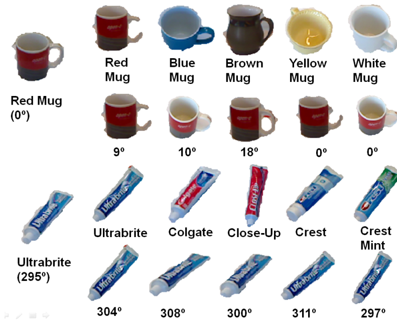
Figure 6.3: Recognition results from the Object-Pose Tree for two objects: Red Mug (top left), and Ultrabrite Toothpaste (bottom left). (Top) From left to right, the top five objects with the highest classifier response at the instance level and at the pose level for Red Mug . (Bottom) Instance and pose classifier responses for Ultrabrite toothpaste .
