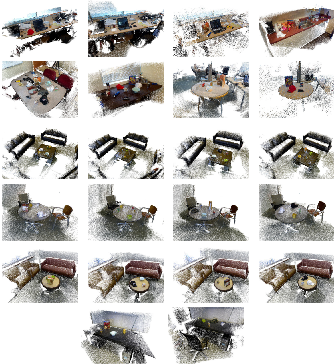
Figure 2.6: The RGB-D Scenes Dataset containing 22 indoor scenes. Each scene is a 3D point cloud created from an RGB-D video. Point-wise ground truth annotations of objects and furniture are available.
