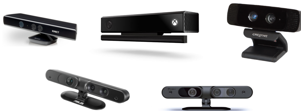
Figure 1.1: Five RGB-D cameras widely available on the market as of 2013. Clockwise from top left, they are: first generation Microsoft Kinect, second generation Microsoft Kinect, Creative Interactive Gesture Camera, PrimeSense Carmine 1.08, and ASUS Xtion PRO LIVE.
