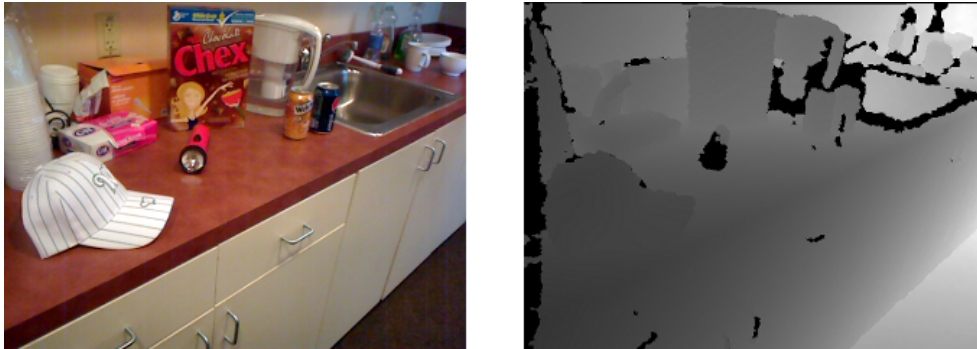
Figure 1.2: An example RGB (left) and depth (right) image pair captured with an RGB-D camera. The RGB image is in true color, while the depth image is in greyscale, where lighter is farther away.
