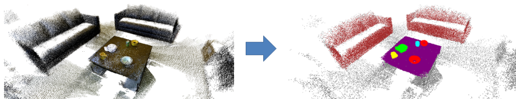
Figure 1.4: Example semantic scene labeling from the RGB-D Scenes Dataset output by the scene labeling MRF described in Chapter 8. (Left) The 3D scene point cloud in true color.(Right) The 3D scene point cloud colored according to semantic label: bowl (red), cap (green), coffee mug (yellow), soda can (cyan), coffee table (purple), sofa (brown), background (grey).
