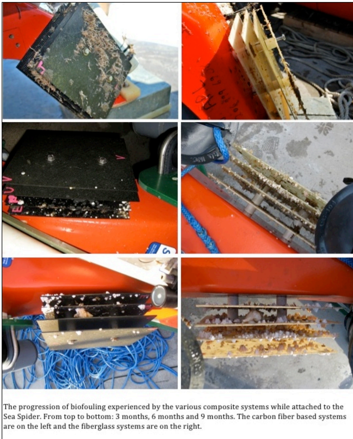
Figure 5-5: Progression of Biofouling Over 9 Months
