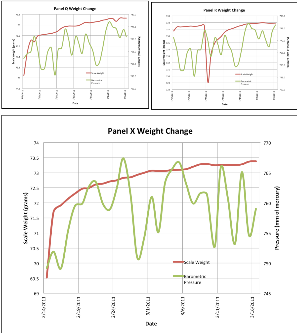
Figure 7-19: The Weight Gain and Barometric Pressure Recorded During Accelerated Exposure for GFRV Panels Q (30°C Exposure), R (40°C), and X (50°C)
