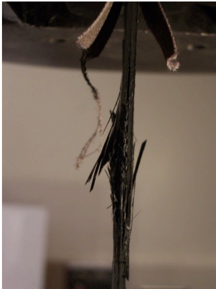
Figure 7-14: Pre-Preg Specimen T1, Seconds Before Final Fracture
