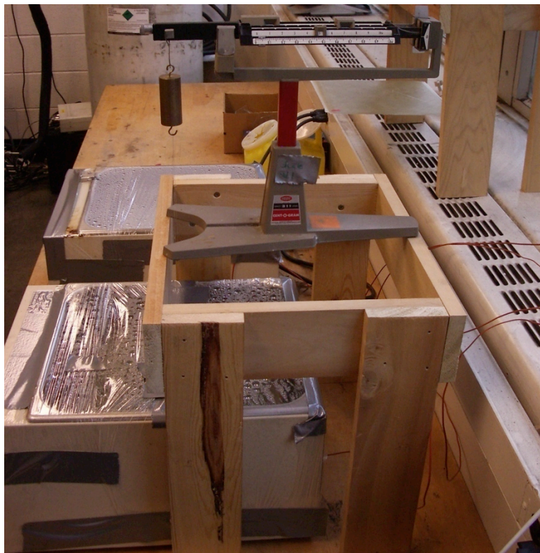
Figure 6-1: Continuous Weighing of Panel Q
