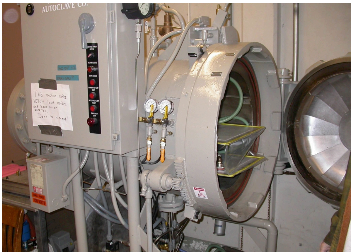
Figure 5-11: Autoclave Used to Cure Pre-Preg Panels
