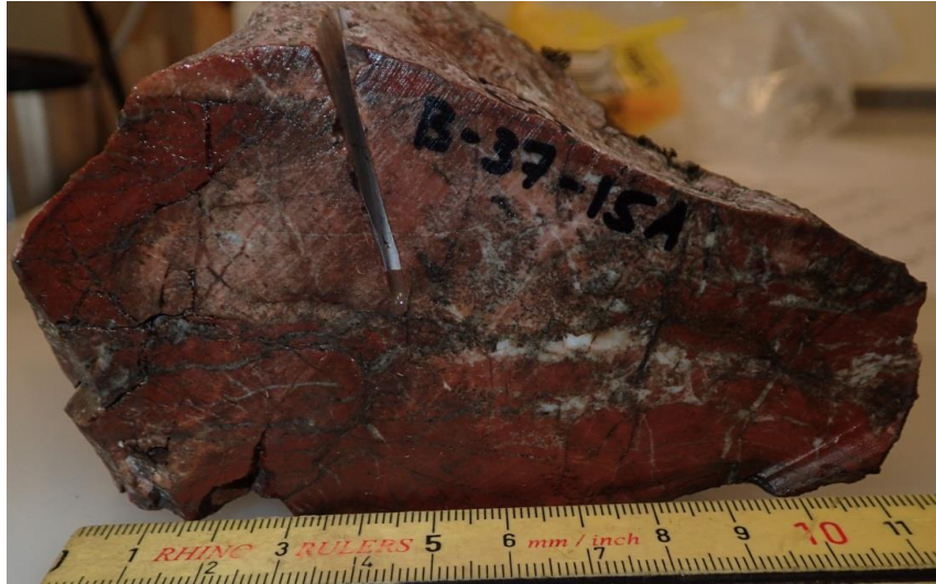
Figure 30 B-37-15A hand sample photo, lighter color – 10R 3/3 (reddish brown), darker color - 2.5YR 3/6 (dark red).
