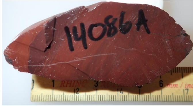
Figure 8 14086A hand sample photo, 2.5YR 2.5/3 (dark reddish brown). Lighter and darker bands are the result of the difference in clastic material abundance as observed in figure 9.
