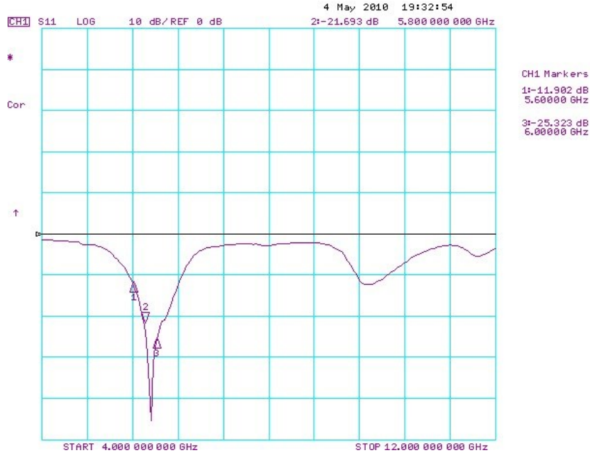
Figure 4.9: Measured |S_{11}| for C-Band slot antenna element in array of 2 WiPAA unit cells.
