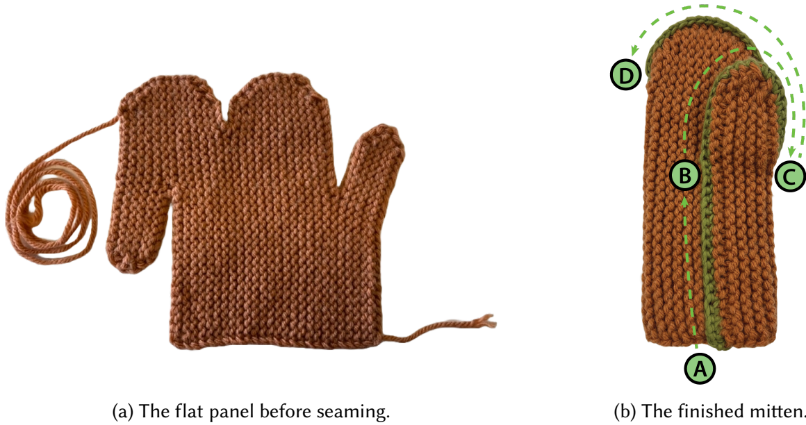
Figure 5.1: The Martha Stewart Cozy Mitten [Martha Stewart Living(2013)]. Knit as a single flat panel (a) and assembled by seaming along path A–D, producing the contrast seam and vertical stitch direction that define the finished object (b). No knitting compiler would choose this plan; PLANEL lets users write it without resorting to machine code.
