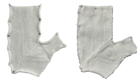
Figure 5.11: Left: Flat-laid mitten panel, illustrating knitting-direction changes between panels. Right: Completed mitten after seaming.
