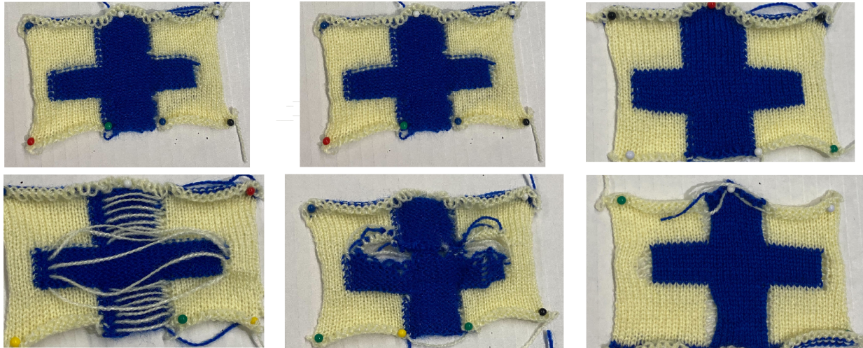
Figure 4.14: Knitting with (top row) and without (bottom row) each contribution. Without float avoidance (left), floats appear on the front of the work. Without path planning (middle), the piece systematically dropped stitches. Without catching (right), the two pieces knit with different colors are disconnected at the vertical edges, leading to the blue sides of the plus sign to curl inwards.
