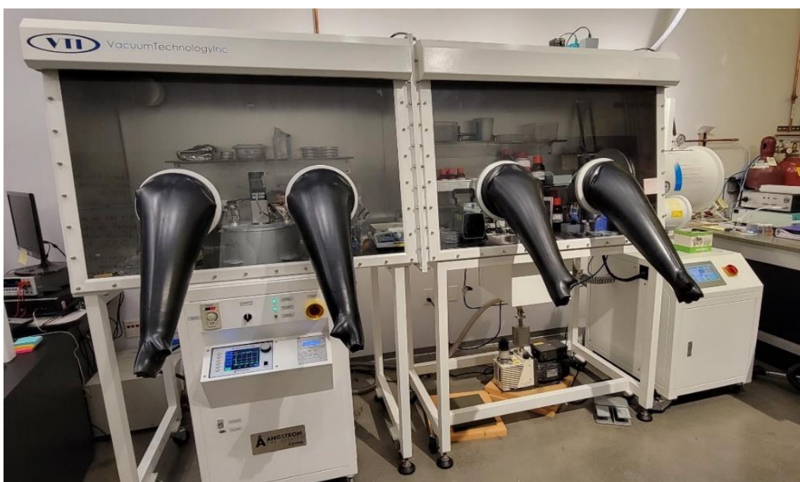
Figure 8: Globe box is used for vapor deposition and other chemical processes.
