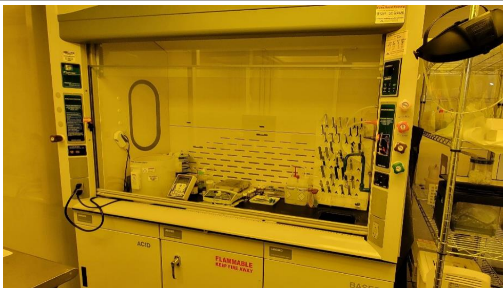
Figure 7: The fume hood in the clean room. Spin coating & annealing is performed in this chamber.
