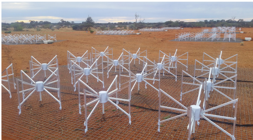
Figure 1.4: The MWA, a radio interferometer in the Australian outback.
