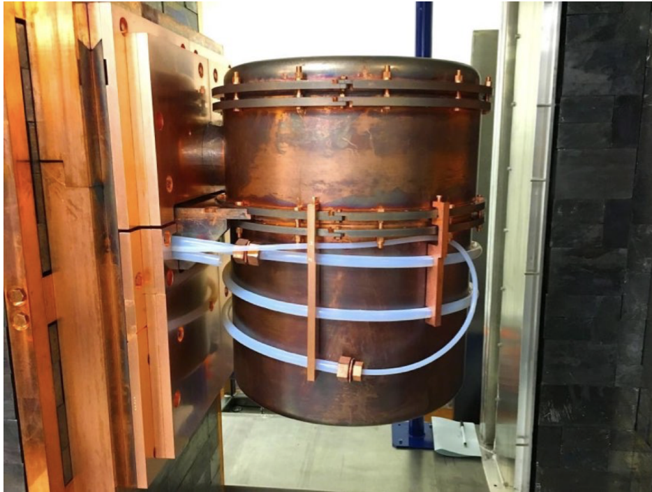
Figure 2.6: A MAJORANA DEMONSTRATOR cryostat. The white tubing is the track used for deploying the calibration source during calibration runs. The cross arm is visible on the upper left of the cryostat, penetrating the shielding structure from the left.
