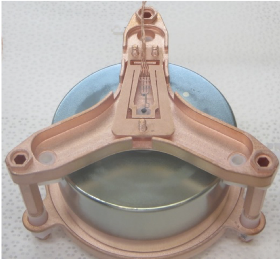
Figure 2.7: Underground Electroformed Copper Detector Holder, with a natural Broad Energy Germanium (BEGe) detector. The low-mass front end (LMFE) is visible near the center of the three-pointed copper structure, held in place by a spring clip. The connector cables are visible towards the top.
