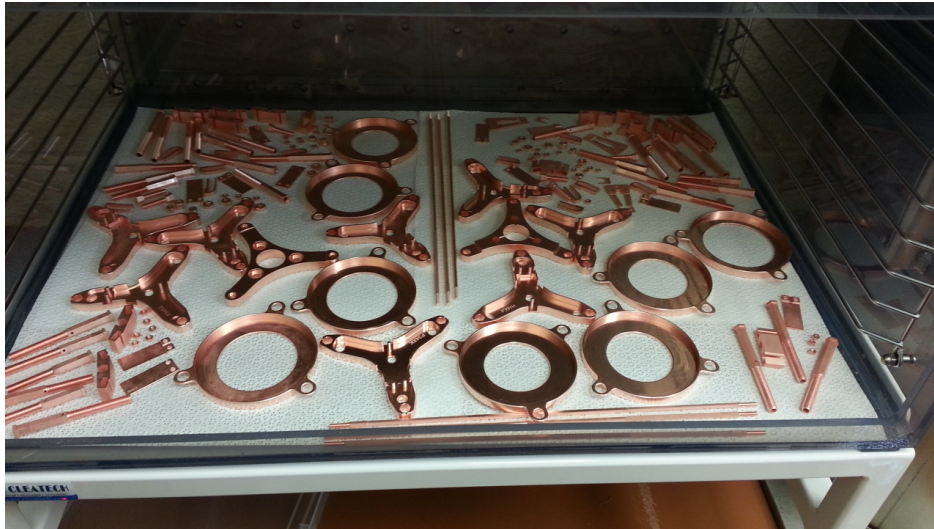
Figure 2.8: Underground Electroformed Copper Parts, held in a nitrogen atmosphere, awaiting the assembly of detector units.
