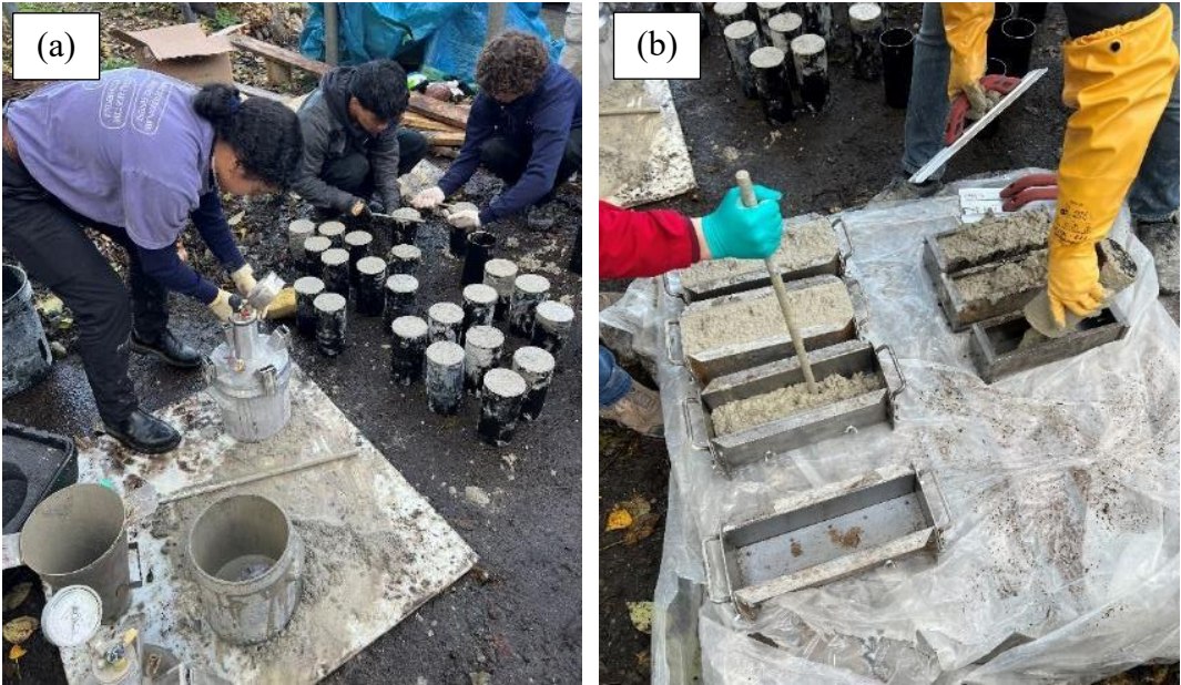
Figure 3-20: (a) Fresh property testing and filling of cylinders, and (b) filling of beams
