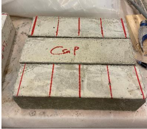
Figure 3-24: Flexural strength specimens marked for the third-point loading method
