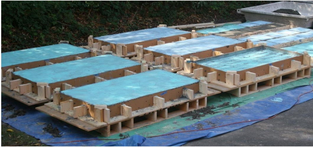
Figure 3-7: Mini-bridge decks with surface retarders applied (Guerrero-Estrada, 2024)
