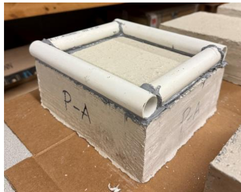
Figure 3-34: Close-up of salt-scaling specimen with dike
