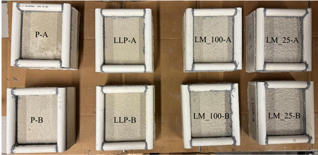
Figure 3-33: Salt-scaling specimens with dikes
