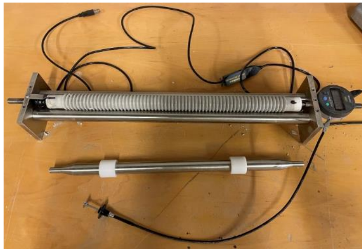
Figure 3-29: Dilatometer bench set up with specimen and reference bar
