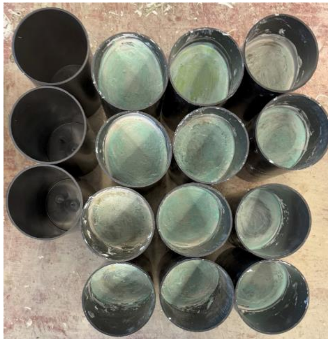
Figure 3-36: Example slant-shear cylinders prepared for substrate casting
