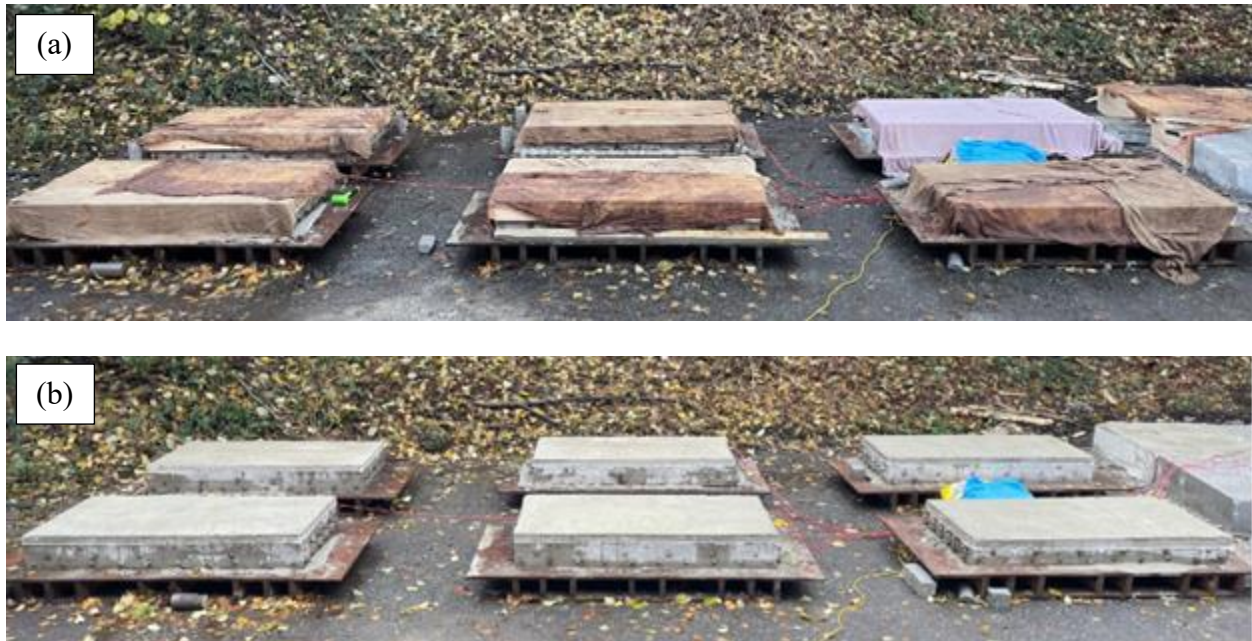
Figure 3-21: (a) The mini-bridge decks curing under burlap, and (b) the decks 24 hours later with burlap and forms removed
