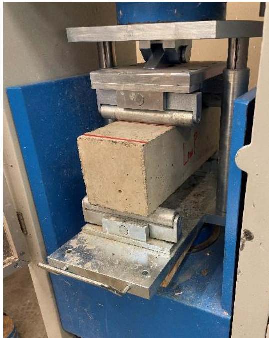
Figure 3-25: Third-point loading method test setup for flexural strength
