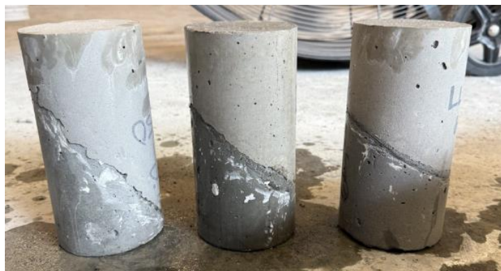
Figure 3-38: Finished cylinder samples at the three different angles, arranged from left to right: 30°, 45°, and 60°
