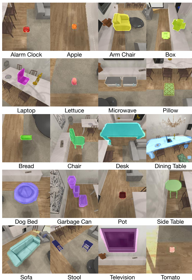
Figure 3.9: MaskRCNN’s qualitative results on 20 used objects. We randomly spawn 20 objects in the testing scene LivingRoom227 and apply the pretrained MaskRCNN to obtain the segmentation results. The object prediction score is set to 0.5 and the segmentation probability is set to 0.1.
