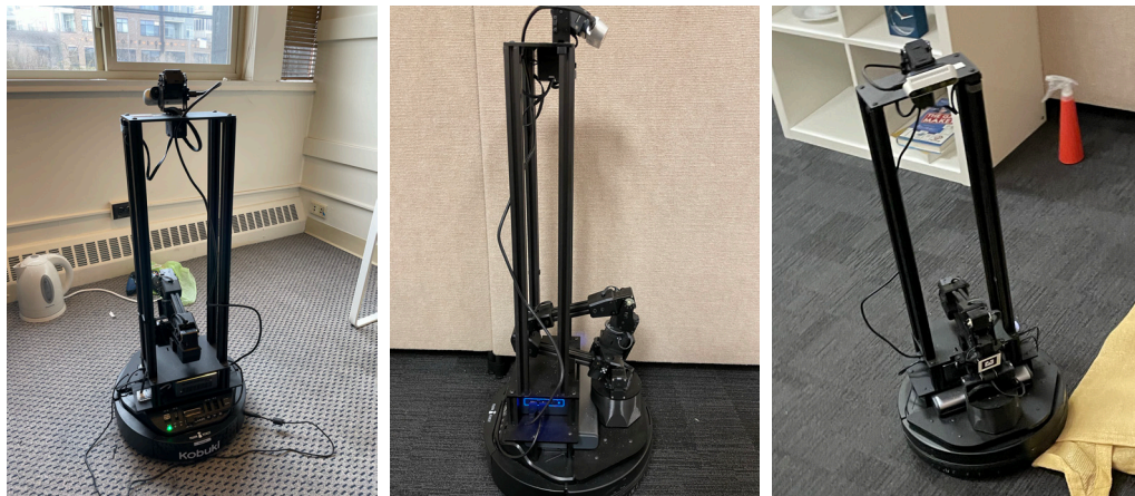
Figure 4.20: LoCoBot. We use LoCoBot from PyRobot [145] with an LQR feedback controller [11] as our embodied agent in the real-world experiments.
