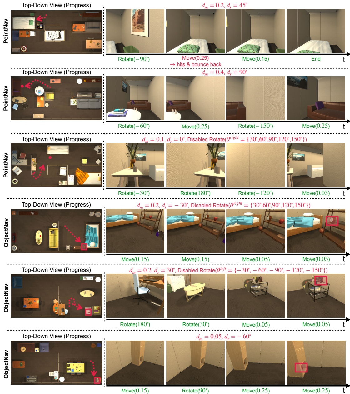
Figure 4.15: Qualitative Results. Examples of PointNav (top tree rows) and ObjectNav (bottom three rows). The agent adapts by rotating in the other direction to compensate for the disabled actions.
